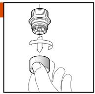
Remove Femco Drain Plug from container, and remove the dust cap.
