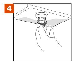
Thread the Femco Drain plug in by hand until snug against the pan. If you meet resistance, back the plug out and try again. DO NOT FORCE the plug into the hole.
