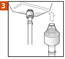
When the Clicker is attached to the Femco drain plug, the valve will remain in the open position.
