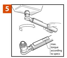
Use a Torque Wrench to tighten the Femco drain plug to the specifications on the container. DO NOT install without using a torque wrench.
