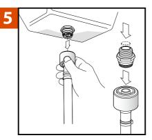
Detach the Clicker by pulling on it. The valve will immediately return to the "closed" position.
