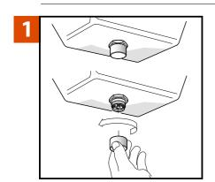
Warm up the engine to operating temperature. Turn off engine. Remove the dust cap from the Femco drain plug.
