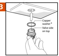
Ensure that the Copper Washer\* is seated on the valve side of the plug (i.e. the top of the plug). \* Copper Washer is not required for plugs in NPT sizes.
