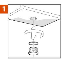
Remove existing drain plug and washer (or oring). Clean the threads in the oil pan. Ensure that the area around the drain plug hole is clean and free of debris.
