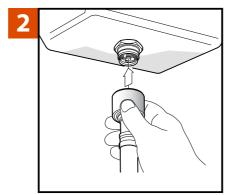
Push the Femco Clicker onto the Femco drain plug.
